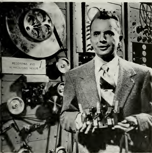
The recording head, which puts signals on tape and provides for video pickup, is held by Joseph Zenel.
