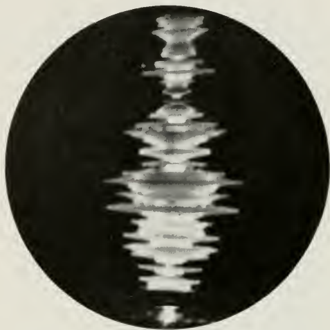
This photograph of the Fischlupe's cathode ray tube shows a school of fish sighted during a test run.
